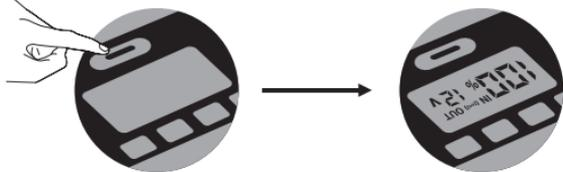
Click button short to step between Voltage 12V/16.5V/19V/24V.
